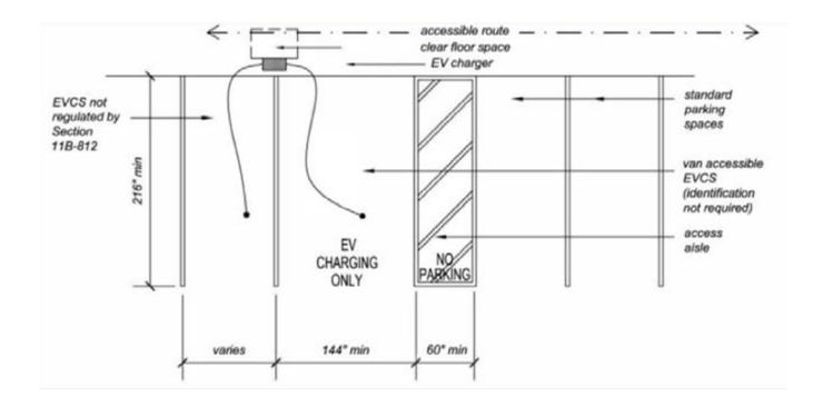
Figure 2: Five EVCS = two accessible EV spaces required
