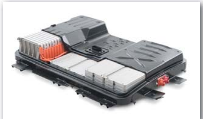
Nissan LEAF battery pack cutaway
